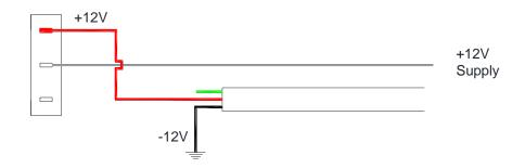
To operate the flash function a double pole ON-OFF-ON toggle switch is required.
