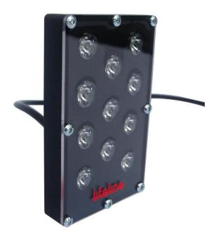
With its high intensity LEDs the new rain light is four times as bright as the previous model. The award winning LEDs themselves are highly energy efficient and have a 35,000 hour lifetime rating. Housed in 6061 Aluminium its robust design will easily meet the demands of a harsh racing environment.
