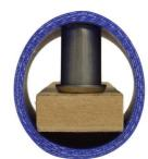
2. Place the hose on a flat surface, using a soft headed mallet, strike the cutting area with a firm straight blow. Carefully remove any excess material with a sharp knife.
