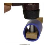
Push the insert through the hole, check thread is clear of any waste material, place pressure sealing washer with lip towards the material and tighten outlet or nut.
