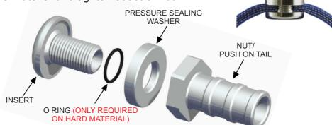
NOTE: Some applications may require the use of PTFE tape to seal the threads
