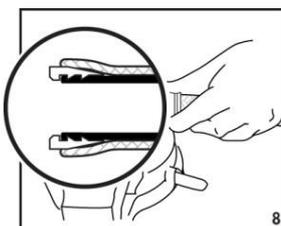
8. Push the hose and sleeve back onto the nipple and bottom against the chamfer. Oil the nipple threads. Start the socket onto the nipple threads and hand tighten.
