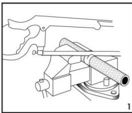
1. Cut the hose to give the required length of hose for the feed and bleed. We recommend the use of a radial wheel but it can be done satisfactorily with a 32 teeth per inch hacksaw blade. In either case, the hose must be tightly wrapped with electrical or masking tape and the cut made through the tape. Do not cut the hose with a chisel, snips, pliers, or a shear as these may crush the PTFE liner.
