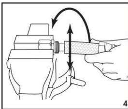
4. Place the hex portion of the nipple in the vice. Insert the end of the hose onto the nipple and bottom the hose against the chamfer seat of the nipple with a rotary motion of the hose. This will size the I.D. of the PTFE tube.
