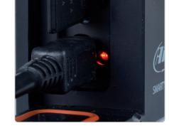
If SmartyCam HD is powered by an external 12V power source or by AiM CAN network a plug icon is shown on the display and the video recorder works in a fully automatic way switching ON/OFF with the external power.
