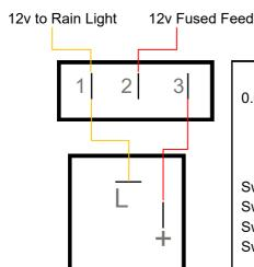
Suitable for Rain Lights drawing between 0.02 and 8 amps. Three position switch allows steady or flashing state.
