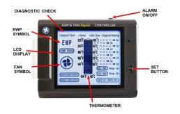
\*Note: This controller (Part No. 8000) is set up for negatively earthed systems however with a wiring adjustment, can also handle positive earthed systems.
