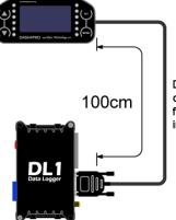
Direct single cable connection for static installations
