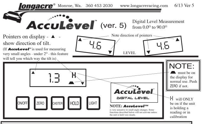
**NOTE:** This Ver. 5 Acculevel<sup>™</sup> has 2 modes of operation. 1) In Normal angle measurement mode the display is steady. 2) In Caster Mode the display flashes (and will not measure absolute angles). Push CASTER button to exit Caster mode and go back to Normal angle measurement.
